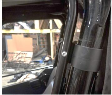
7. Attach both Large Hole Plastic P Clamps (H) to the Inner Subframe (B) using the M6x35mm button head bolts and locknuts. Do not fully tighten at this time. The Inner Subframe (B) will be adjusted in a later step.
