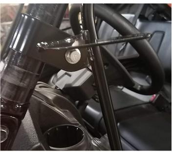
**4.** The Front Hinge Clamp (F) Must be installed as shown in the image above with the Inner Subframe (B) tab **sandwiched** in between the clamp ears.
