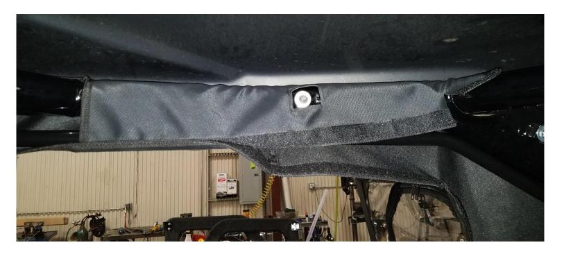
**24.** Moving from the top right corner along the roofline, wrap the Inner Subframe Textile (E) around the ROPS and Inner Subframe (B) as shown in the pictures above and below. Make sure the bolt head lines up with the square hole in the textile flap. This will ensure alignment of the textile is close. Final adjustments will need to be done once the Inner Subframe Textile (E) is attached at all spots.
