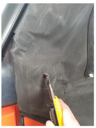
**41.** Using a sharp razor or utility knife, cut the textile so the mirror mounting bolt can pass through.
