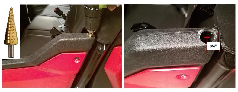
**8.** Starting with a 1/8" pilot hole, drill a hole in the top surface of the door with the center 3/4" from the rear edge as shown in the images above. Increase the hole to the final 5/8" size (a step bit works well, but a standard bit may be used).
