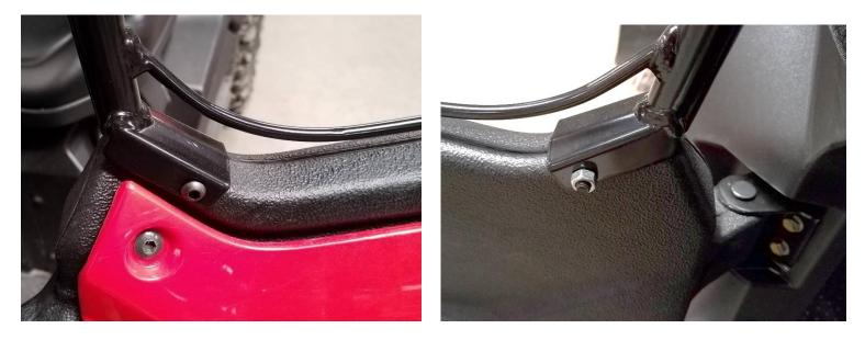
**11.** Install Upper Door Frame (A) front mount using supplied M6x40mm bolt and locknut as shown in the images above.
