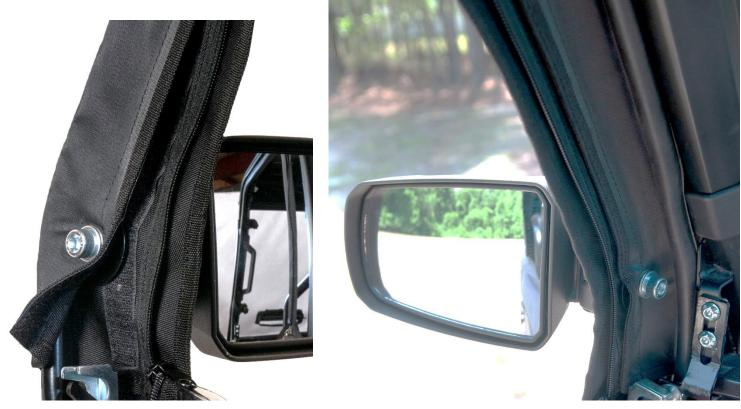
**42.** Pass the bolt through the mounting bracket and thread into the mirror and tighten (DO NOT OVER TIGHTEN).
