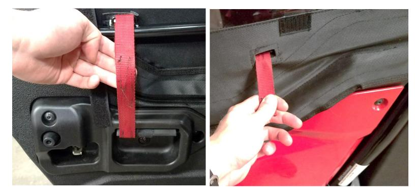
**39.** The door can now be opened using the pull strap. From the inside the strap makes a loop that can be pulled to actuate the door handle. From the outside, simply pull the tab and the door should open with minimal effort. See above images.
