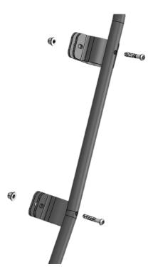
**6.** Position the remaining 2 Large Hole Plastic P Clamps (H) around the rear ROPS structure with the ears towards the inside of the vehicle as shown. Line up with the holes in the rear of the Inner Subframe (B).
