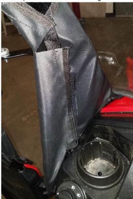
**31.** Finish wrapping the large triangular section of the Inner Subframe Textile (E) around the ROPS and Inner Subframe (B) as shown in the image above.
