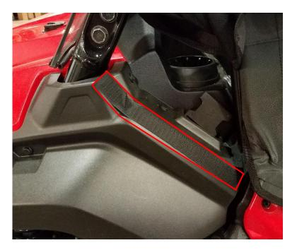
**28.** Before moving further, a 10" piece of adhesive Velcro needs to be applied above the front fender in the area shown. For best adhesion, it is highly recommended to clean surfaces with alcohol or degreaser before applying adhesive Velcro.
