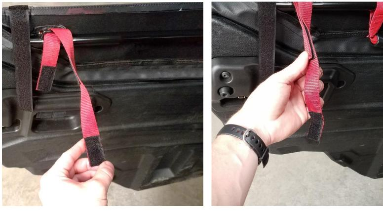
**37.** Moving to the inside of the door, make sure the upper part of the strap is attached to itself with Velcro. This ensures the strap can be used to release the door from both the inside and outside of the vehicle.
