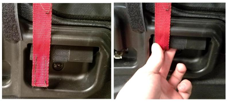
**38.** The strap is secured to the handle using Velcro. Wrap the strap to the face of the handle and up underneath to ensure there is good Velcro adhesion. See above images.
