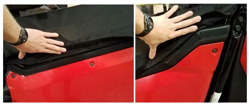
**33.** The Upper Door Textile (D) needs to be secured to the Honda lower door using a 35" piece of adhesive Velcro. The Velcro is to be applied to the black plastic above the color panel as shown in the image above. . For best adhesion, it is highly recommended to clean surfaces with alcohol or degreaser before applying adhesive Velcro.
