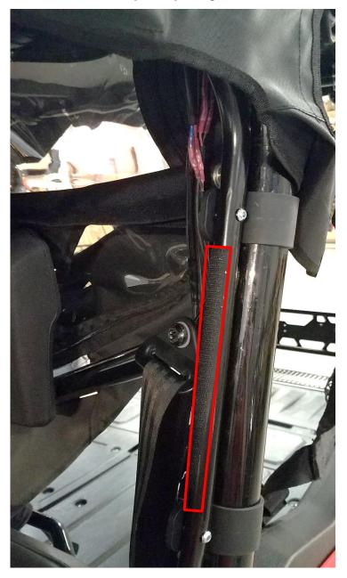
**20.** Next place a 9" piece of adhesive Velcro on the Inner Subframe (B) between the 2 rear clamps in the postion shown in the image above. For best adhesion, it is highly recommended to clean surfaces with alcohol or degreaser before applying adhesive Velcro.
