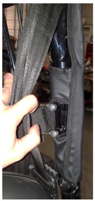
**23.** There are 2 flaps at the bottom of the rear section of Inner Subframe Textile (E) that need to be secured around the ROPS and Inner Subframe (B) as shown in the image above.
