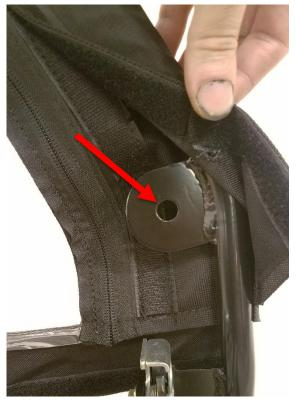
**40.** Locate the mirror mounting bracket on the inside of the door frame. Mark the location of the hole with a punch so that it can be seen on the outside of the door textile.
