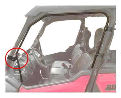
**1.** The first step is to install the Inner Subrame (B) onto the vehicle ROPS. This is done using 3 clamps on each side. The first clamp to install is (F) the Front Hinge Clamp.
