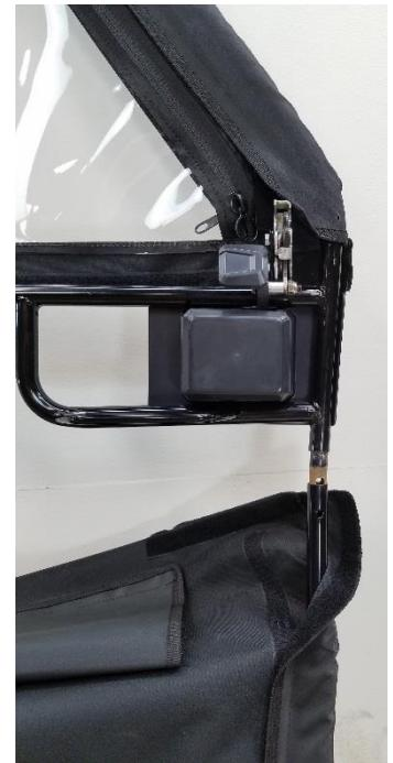
**7.** Align Door frames, ensuring the two pieces are the same side (Both Driver sides, or both Passenger sides. Driver Door shown) and join the two door halves together. It will help to detach some of the Velcro on the lower door frame in order to make access to the tubing easier.
