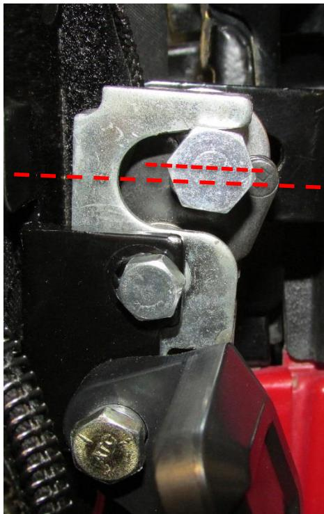
**27.** In the image above the striker is aligned incorrectly. Note the latch is not fully closed and the striker bolt is not aligned in the center.
