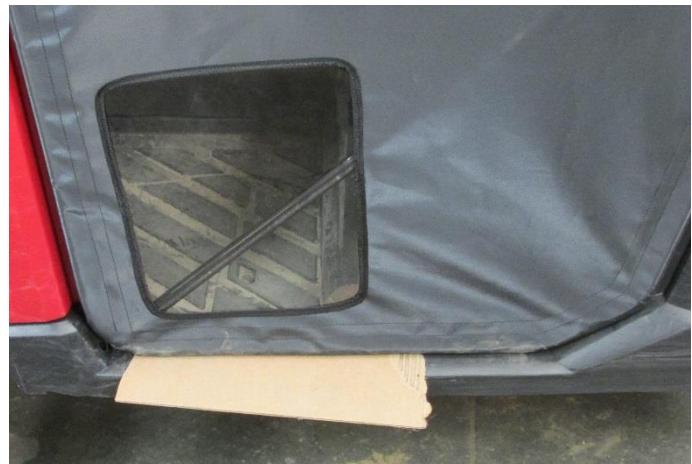
**20.** Move the door into the “closed” position. With the window down, you can make adjustments to the striker bolt and plate to ensure the door fits properly.
