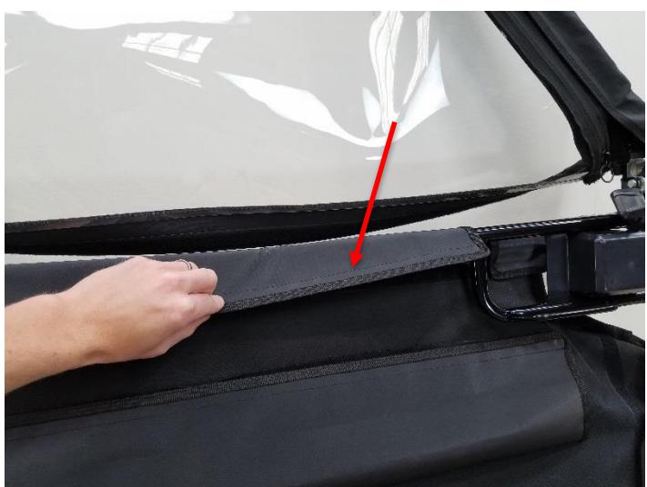
**9.** Pull upper rear flap from lower door panel snugly over the door arm bar and secure flap to hook Velcro.
