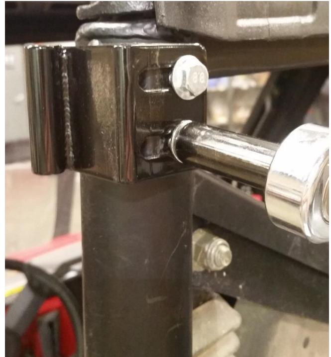
**30.** The Upper Hinge mount plate may be adjusted in and out to affect how much the door will compress the gasket.
