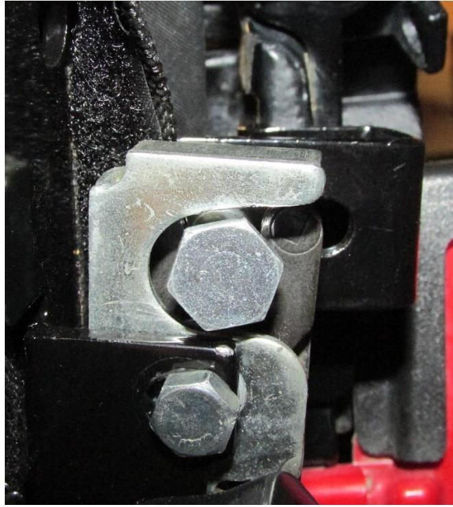
**26.** Shown above is the correct alignment for the striker bolt and latch when the door is fully closed.
