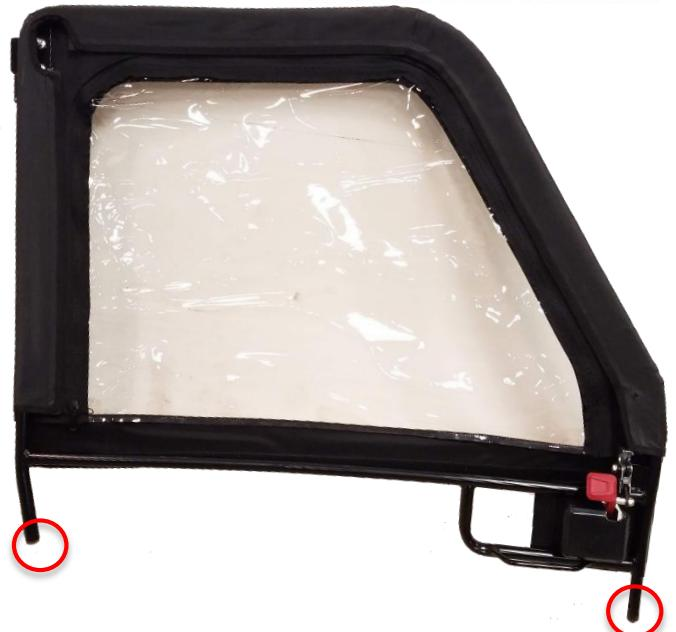
**6.** Locate attachment locations circled on both the Lower and Upper Door Frames. The sleeve tubing in the Upper door frame will slide into the tubing of the lower door frame.
