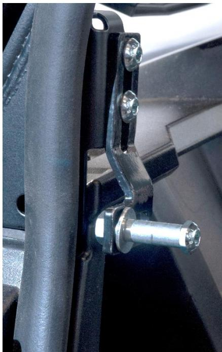
**4.** Move to the front corner of the ROPS structure. The Striker Plate will be installed using M8x20mm fasteners and M8 Washers in the holes provided on the ROPS structure as shown. (note these holes are slotted for striker adjustment. Do not fully tighten at this point.)
