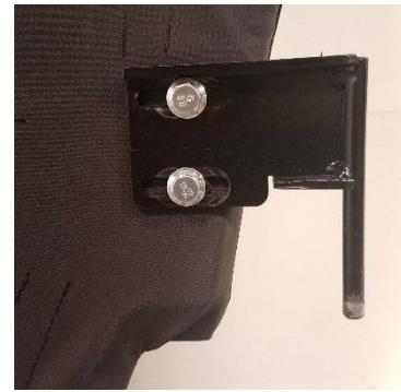
**17.** Pass M8x25mm bolts through the Upper Sliding Hinge, textile, then the welded on door plate. Attach using M8 washers and lock nuts as shown. Repeat steps for Lower Sliding Hinge using M8x25mm bolts, M8 washers and lock nuts. Do not fully tighten at this time. Sliding Hinges are slotted for door adjustment.
