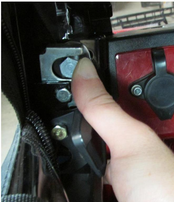
**22.** With the striker bolt loose and door pressed firmly against the body work and gasket, move the striker bolt into the closed position of the rotary latch. There should be two clicks when it is fully latched. Note the location of the striker bolt on the striker plate. This will give you a good starting point for adjusting the door.
