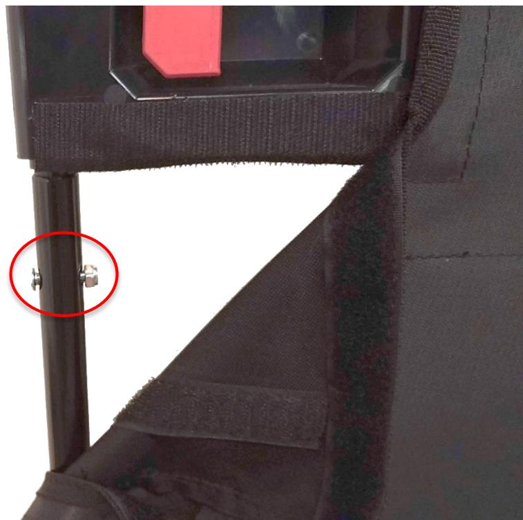
**8.** Attach Upper and Lower door frames using M6x25mm button head fasteners and corresponding M6 locknuts. The locknut should be on the inside of the door frame as shown.
