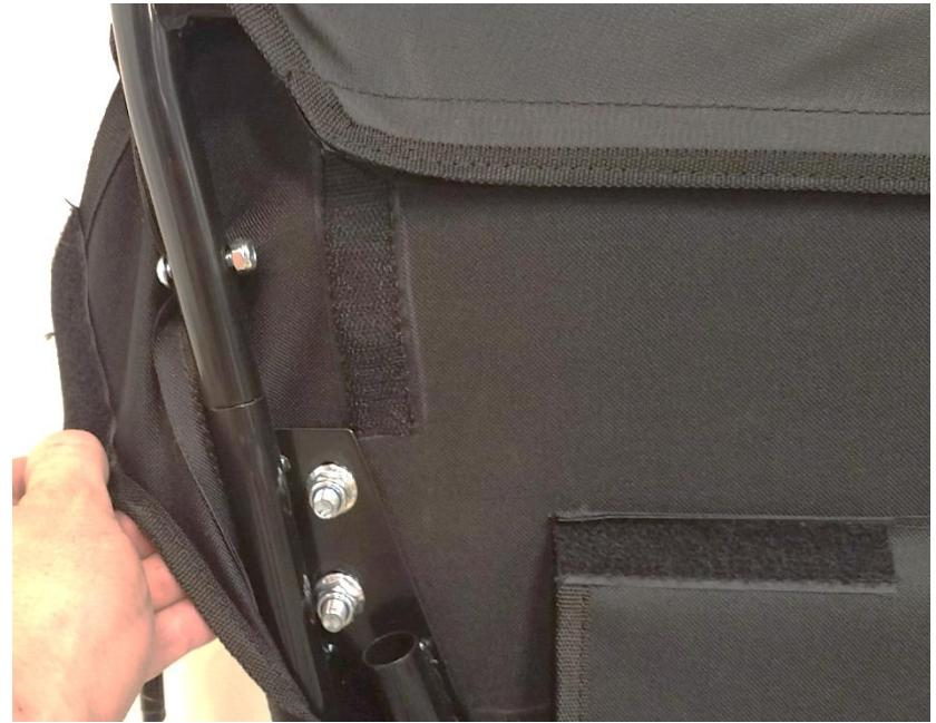
**11.** Continuing down the door, attach long flap at the forward section of the lower door tubing to the hook Velcro on the inside of the panel.
