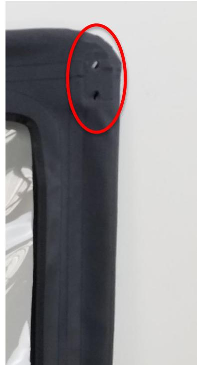
**16.** Holes need to be cut in door textile panels in order to mount the Upper and Lower Sliding Hinges. **Ensure textiles are tight and fit as desired before marking and cutting holes.** Take a sharp scribing tool and punch a small hole through the textile indicating the center of the slot. Take a razor blade and carefully cut out the small amount of textile so that the supplied M8 bolt may pass through the plate and the textile. Repeat this process for the lower mounting location.
