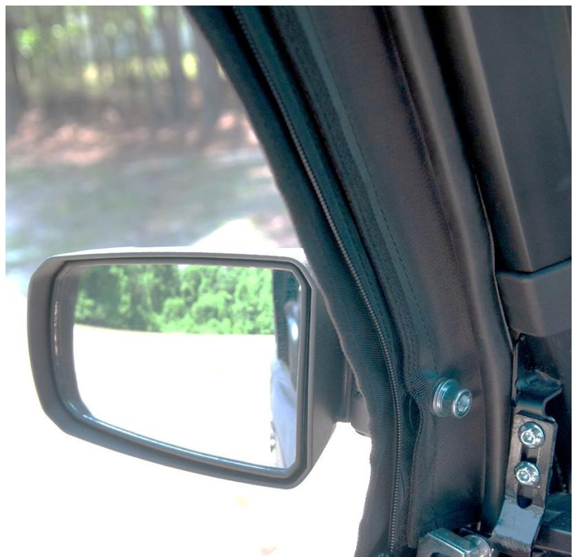
**34.** Pass the bolt through the mounting bracket and thread into the mirror and tighten (DO NOT OVER TIGHTEN).
