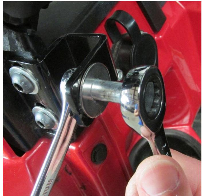
**23.** Open the door and tighten the striker bolt to the plate. Leave the two bolts attached to the ROPS structure loose so that the assembly may move up and down.
