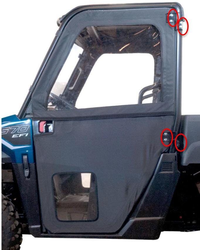
**31.** Once the door has been adjusted as desired, fully tighten down all fasteners on door hinge sliding plates, and hinge mounts. Before operation, ensure all Velcro is securely fastened.
