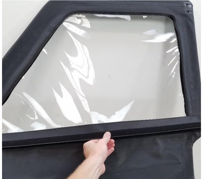
**14.** Pull Upper door textile down firmly and attach to loop Velcro located on the outside of the lower panel as shown.
