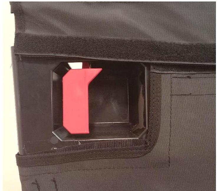
**15.** Pull Upper door textile and align the Velcro so that it attaches to the plastic molded pocket without obstructing handle movement.
