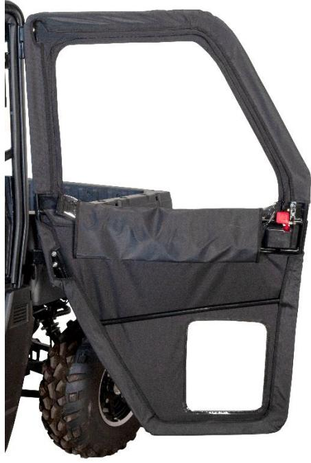
**19.** Insert the Sliding Hinge Pins into the Hinge Mount Barrels and roll down the window for easier adjustment. Rolling down the window will allow you to access and adjust the striker bolt and plate from the outside of the vehicle.
