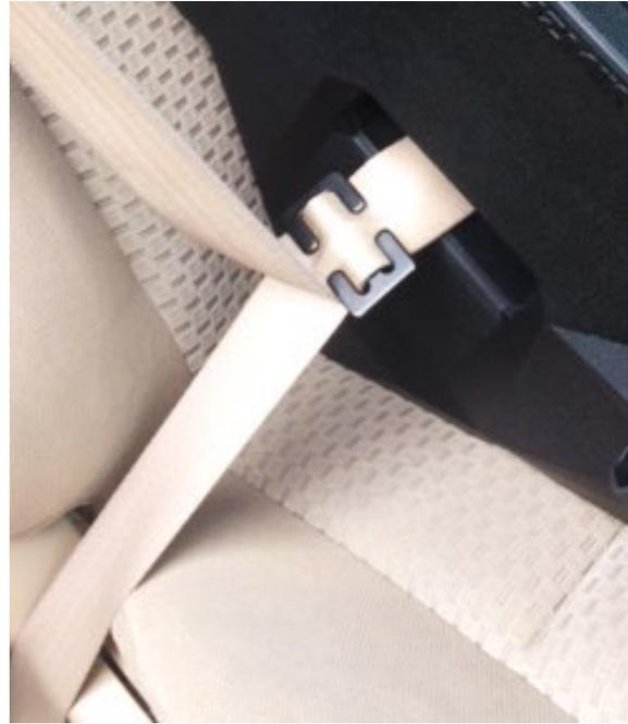
5. Place the assembly on the vehicle seat. Run the seat belt through the middle hole and buckle into the seatbelts receptacle. Pull the loose tab to get the seatbelt as tight as possible. For 3 Point seatbelts, use supplied seatbelt clip as shown in the above right picture to secure the belt.
