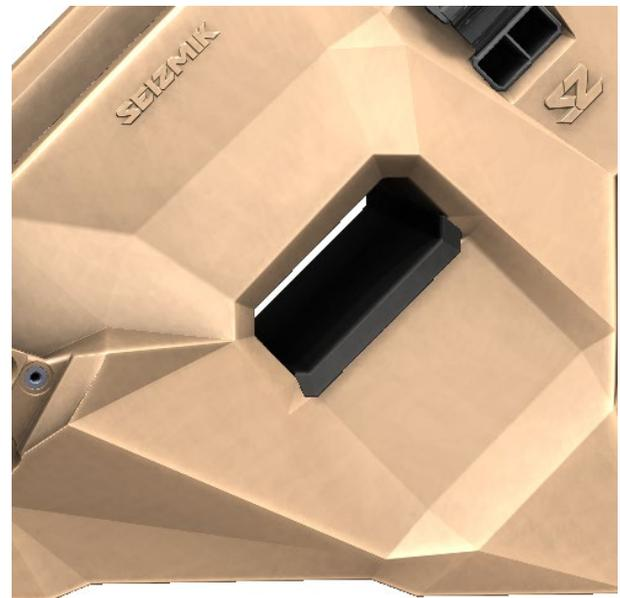
2. When installed, the seatbelt insert should lay flush and match the style lines of the foam base.
