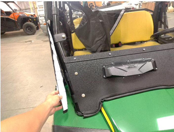
3. Peel back the adhesive strip.
