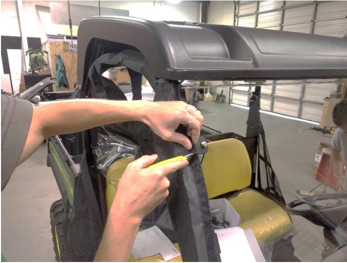
1. Make two careful cuts in the textile at the bottom and top of the upper P clamp.
