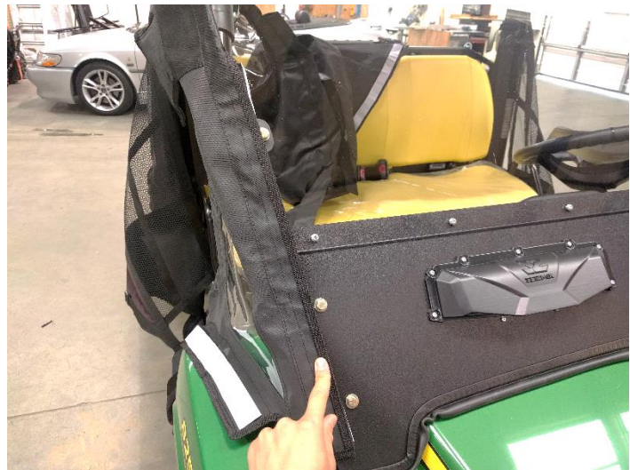
4. Adhere the textile to the front of the windshield.
