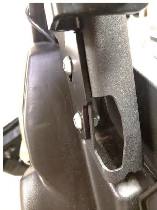
12. Pass M8x16mm button head bolts through the Striker Bolt Mount Plate (K) and front stamping on the Defender ROPS. Attach using M8 flange bolts and lock nuts as shown. Do not fully tighten at this time. Plate is slotted for door adjustment.
