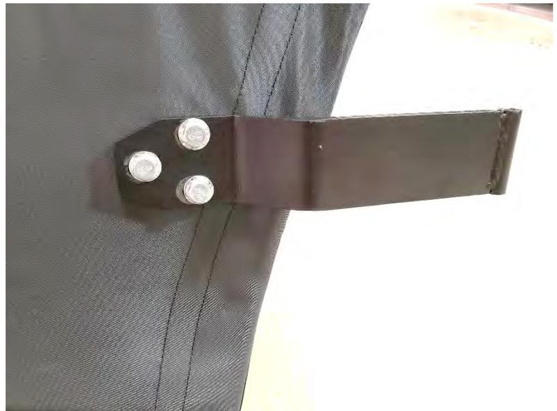
11. Pass M8x25mm flange bolts through the Lower Door Hinge Plate (G), textile, then the welded on door plate. Attach using M8 flange bolts and lock nuts as shown. Do not fully tighten at this time. Hinges are slotted for door adjustment.
