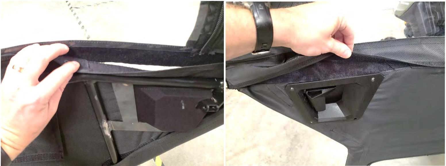
7. Pull the lower textile upwards and the upper textile downwards to line up the 2" seam Velcro so that the textile is snug and lines up evenly.
