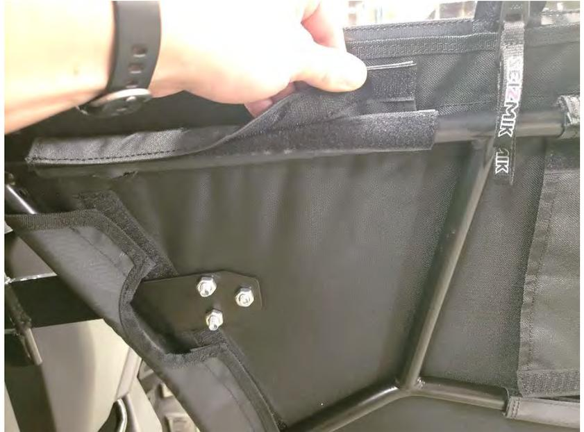
4. The upper and lower textiles come on each half of the frame but you will need to attach the halves together and ensure they are properly secured. The highlighted areas are the main areas you will need to address. There are 3 center flaps that wrap around the tubing along with the 2" Velcro seam between the upper and lower textiles.
