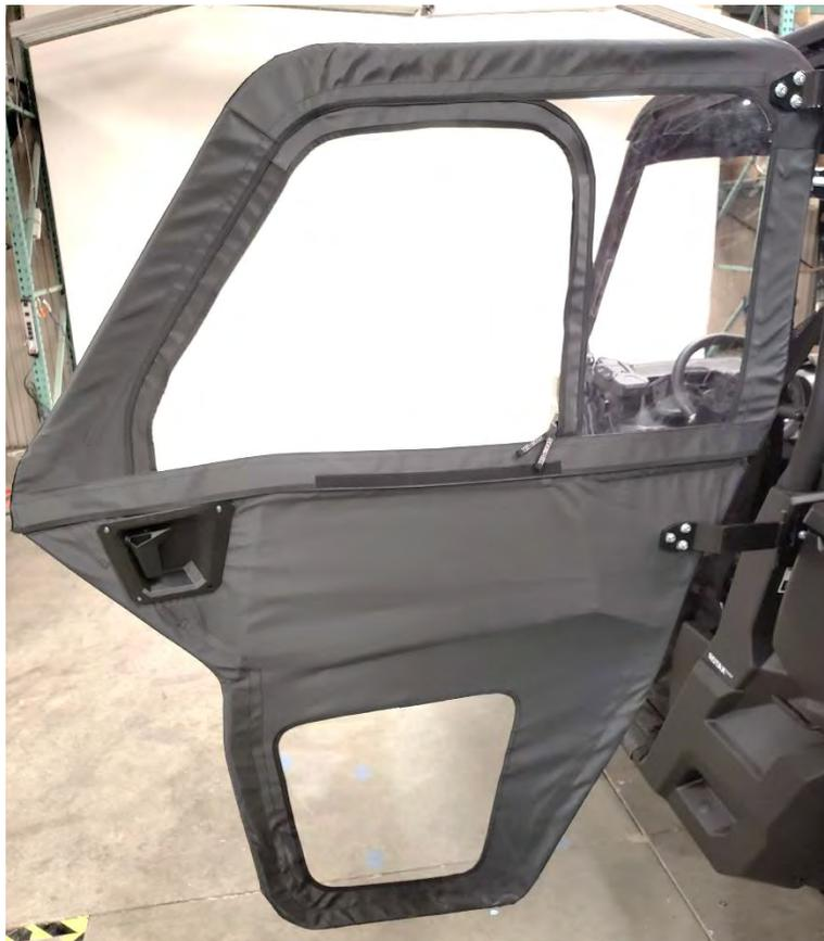
8. The textiles should appear taut but not bursting at the seams. If they are too tight in warmer weather, they will only become tighter in cooler temperatures. If you are installing these doors in the summer, give yourself some slack in the textile fit-up so that when winter rolls around, the textiles will fit properly.
