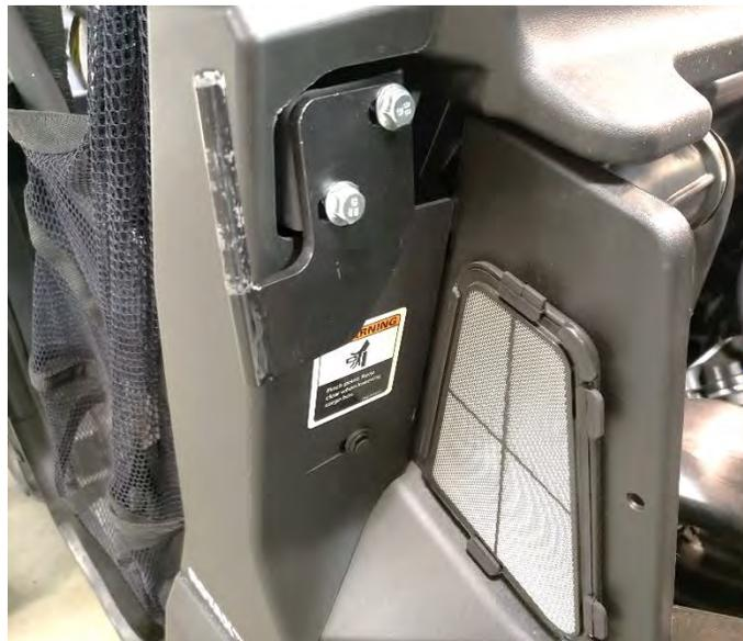
2. Locate the lower 2 threaded holes at the back of the cab. It will make it much easier to access if you tilt the bed back. Install Lower Door Mount (I)\* using 2 M8x16mm flange head bolts. Snug the bolts down but do not tighten all of the way. You will need to adjust them later once the door is on.
