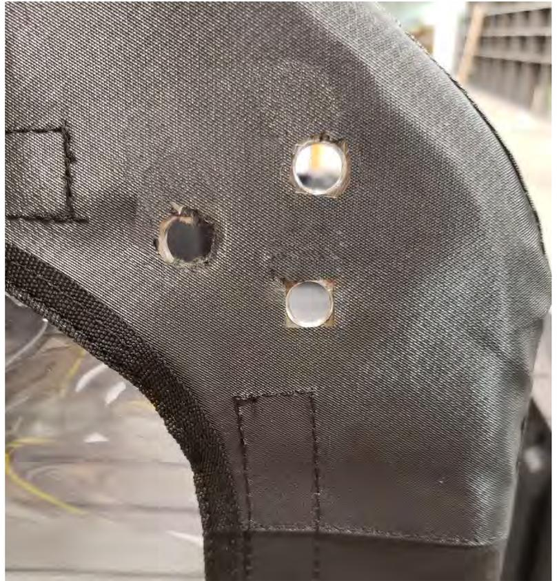
9. Holes need to be cut in door textile panels in order to mount the Upper and Lower Sliding Hinges. **Ensure textiles are tight and fit as desired before marking and cutting holes.** Take a sharp scribing tool and punch a small hole through the textile indicating the center of the slot. Take a razor blade and carefully cut out the small amount of textile so that the supplied M8 bolt may pass through the plate and the textile. Repeat this process for the lower mounting location.
