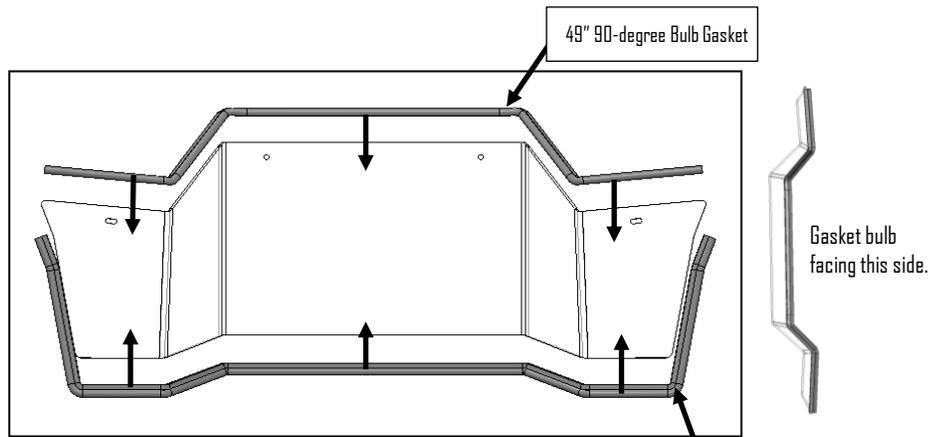
2. Push 49" 90-degree bulb gasket onto lower windshield with the bulb section oriented as shown. Push 63" 180-degree Bulb Gasket onto lower windshield.
