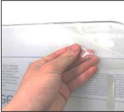
1. Peel plastic 4" back on edges of windshield. Remove completely after windshield is fully installed.
