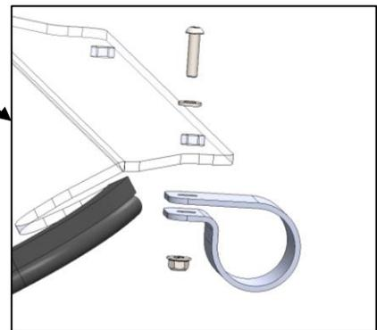
6. Insert bolt through washer and windshield, loosely install nuts on both top clamps.
