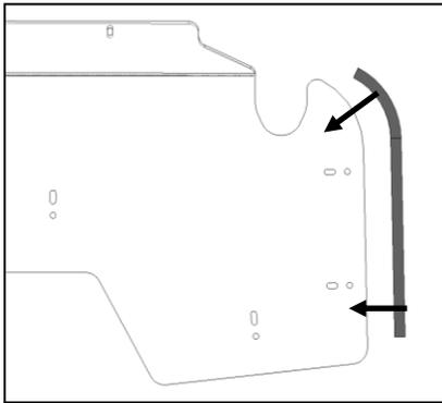
3. Push the 13.25" gaskets on the upper windshield with the bulb section oriented as shown.
