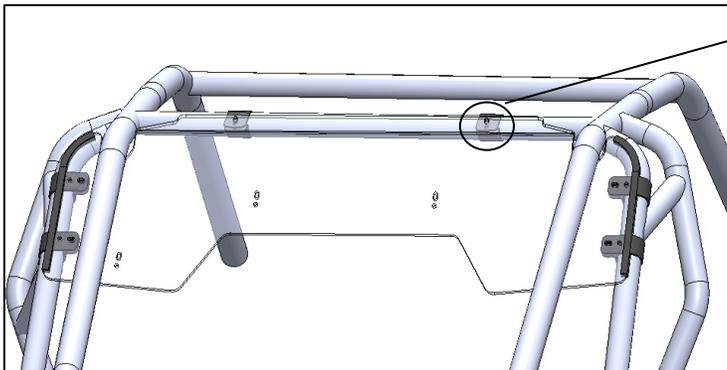
5. Place upper windshield in location shown. Gasket bulb should be against roll cage.
